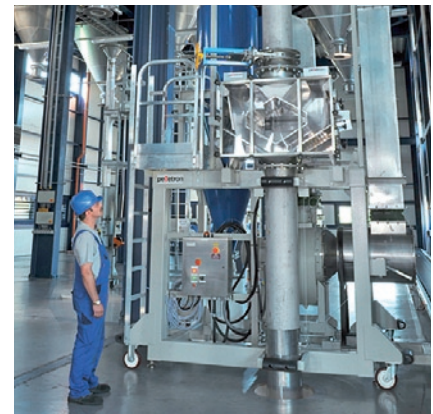
DeDuster ® – System in loading position
